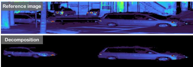
Figure 12. Decomposition results on Waymo dataset [40]. The points are colorized by intensity values from blue(0) to red (1).
